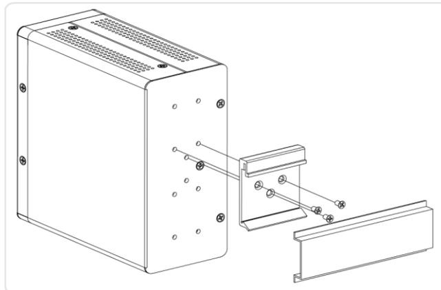
**Figure 3: Screw DIN Rail Kit to the Switch**
