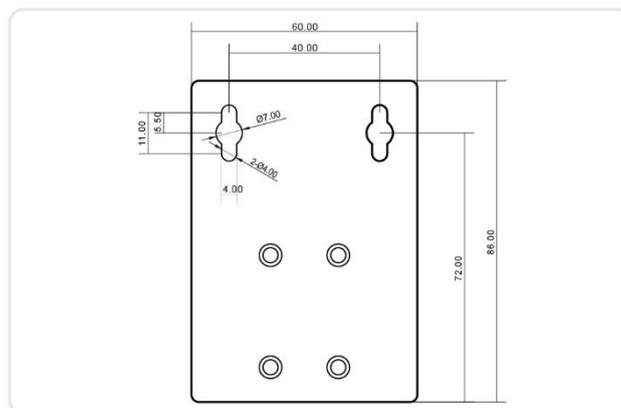
**Figure 7: The Dimension of Wall Mounting Plates**
