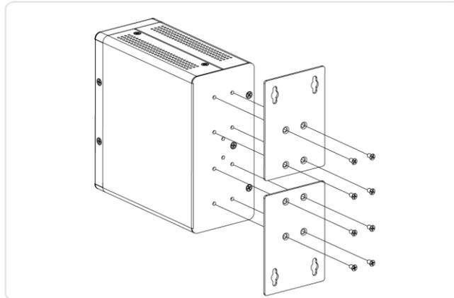
**Figure 6: Attaching Wall Mounting Plates to the Switch**
