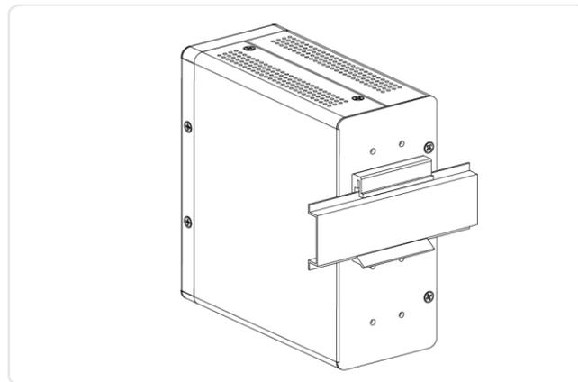
**Figure 5: The switch is fixed to DIN Rail**
