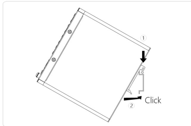
**Figure 4: Clip switch to the DIN Rail**
